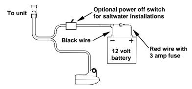
Power and transducer connections for the Cuda 250 sonar units (direct battery connection shown).
